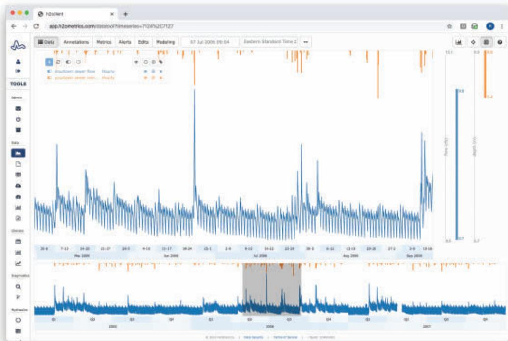
This figure shows an example of the type of data that should be collected from a sewer system. The flow is the blue line, and the rain is the orange line. H2Ometrics
